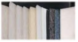
Recycled textile fibres, recycled PET fibres and / or sheep wool non-woven type of thermo-insulating products.
