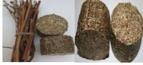
The crop residues (stalks) had moderate gross calorific value of 18.4 MJ/kg, the briquettes have specific density 916 kg/m3, were very solid and were not cracking.
