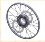
Figure 2. Spatial view of a bike wheel with the electric machine incoporated
