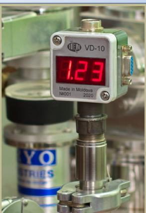
orinciple of operation of deformation vacuum gauges is based on the deformation of flexible structural elements of the transducer owing to pressure difference. The main advantage of deformation instruments is that the pressure readings are independent of the gas type. This feature is particularly important in view of the increasing number of applications of ionplasma technological processes that occur at pressures of a few Torr.
