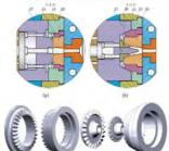
Fig. 2. Local sections of the mold forming knot: (a), (b) - for the manufacture of fixed and movable central wheels of the ZK-H precessional gear respectively; (c), (d) - 3D views of fixed center wheel and mirror profile die; (e), (f), (g) - respectively the views of the central movable wheel, the reinforcement and the mold with mirror profile.
