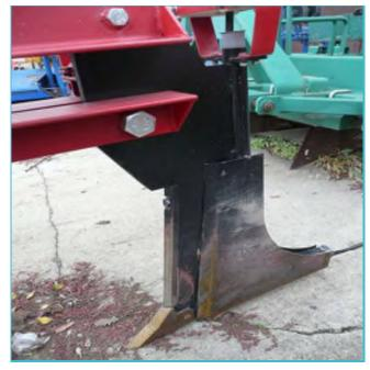
The technical problem solved by the proposed solution is the mounting system of the active part, which facilitates the rapid change in the field, either of the knife, or of the blade, or of the knife-blade assembly, depending on their degree of wear.
