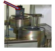
The two magnetrons of the sputtering equipment used to obtain TCO layers, which improve with RTA.
